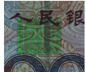
IR 740 - 1100 nm illumination for «anti-Stokes inks» examination
